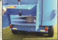
Rubber Side Extensions are 9-1/4" high and add additional mixing capacity.
