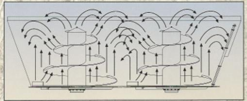
Feed is pulled away from the bottom of the mixer walls by the specially designed screws, allowing more material to fall as the screws rapidly lift the feed. The continuous lifting and falling action creates a thoroughly blended mixture of ingredients within a few minutes.
