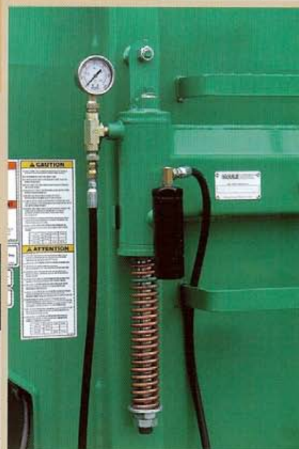
Master cylinder and pressure regulator of the disc brake system
