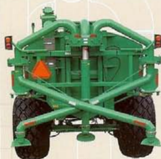
Mechanical Articulations without Flexible Hose
